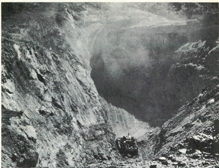
Bulldozer stripping hanging wall of Barite seam, S.A. Barytes, Oraparinna
